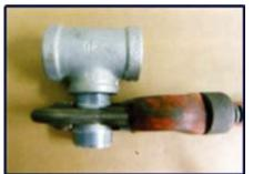
Disconnect the Nipple from the Flexible Sprinkler. Connect the Nipple to the main piping with normal sealing procedures and tighten using a pipe wrench to ensure a leak-proof connection. Do not over tighten. Connect the Flexible hose to the Nipple by finally tightening the nut. Make sure gasket and isolation ring are properly located at the end of the Flexible hose before connecting the hose to the main piping system
