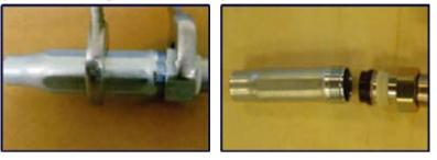
Disconnect the reducer by turning the Nut (not the Reducer) from the Flexible Hose.
