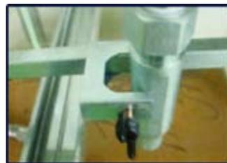
Insert the reducer from the side of the center bracket in a horizontal direction (not from the top vertically). Adjust the angle of the reducer by turning it gently into the bracket.
